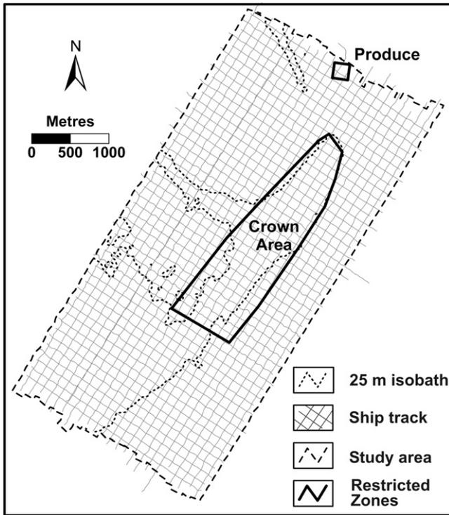
Fig. 3. dGPS tracklines showing data coverage in the survey area. Also shown are the Produce and Crown Restricted Zones of the MPA and the 25-m isobath, which was used to delineate the Crown Area Restricted Zone.
