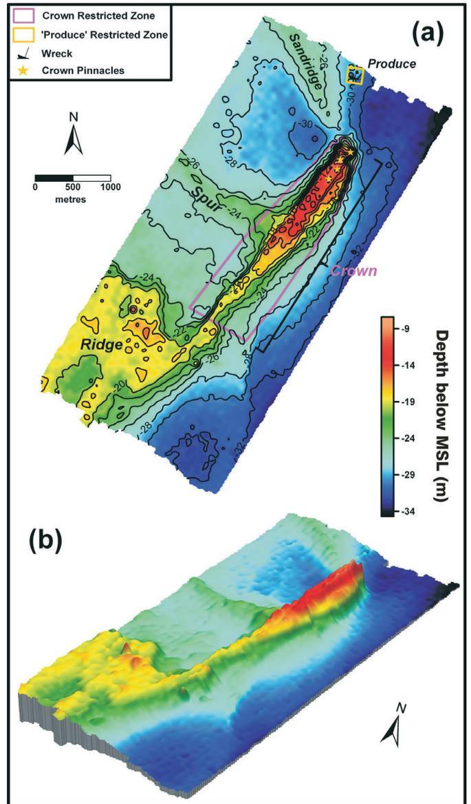
Fig. 4. (a) Bathymetric contour map of the study area showing the main morphological features and the boundaries of the Restricted Zones of the MPA. Contour interval is 2 m. (b) 3-D bathymetric model of the study area; view is from the south, sunshading from 150° with a 75° azimuth.
